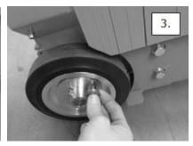
Disengage Mode (Pic 2), allows the machine to be moved around freely not under power.
